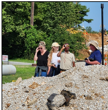
NRCS Pathway students, Racheal Voss and Dee Harris, (2nd and 3rd from left) use the clinometer to measure the angle of slope.
